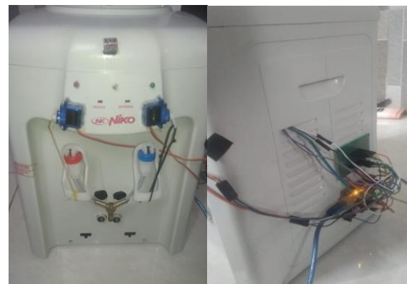
Figure 11. Automatic water dispenser based on gesture detection.
