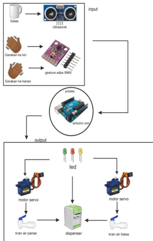
Figure 4. System architecture design.
