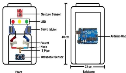
Figure 3. Mechanical system design.
