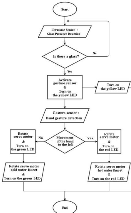
Figure 10. Software design flowchart.
