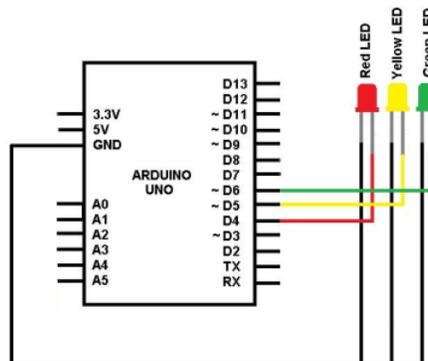
Figure 7. Schematic of the LED module circuit.
