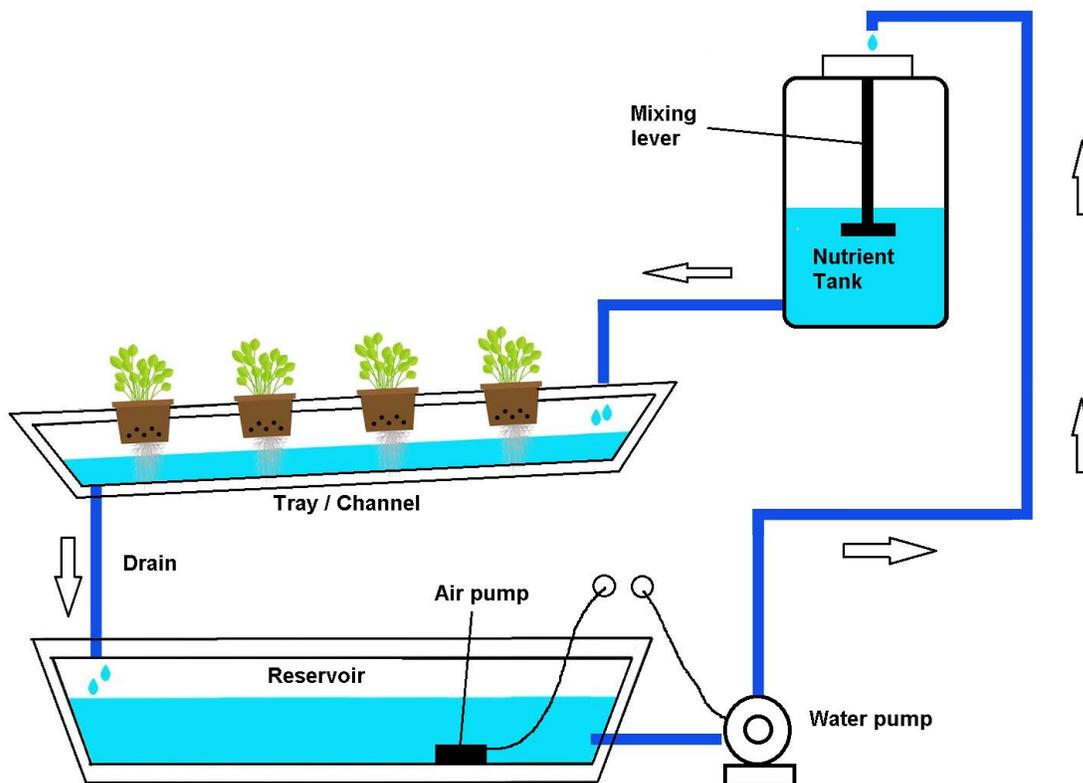
Fig. 1. Schematic Diagram of Hydroponic NFT Installation
