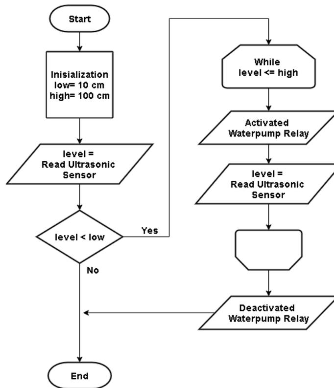
Fig. 5. The Flowchart of Nutrient Distribution In The Hydroponic System.
