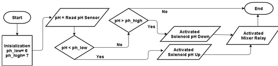
Fig. 4. The Flowchart of The Hydroponic Nutrient PH Regulator.
