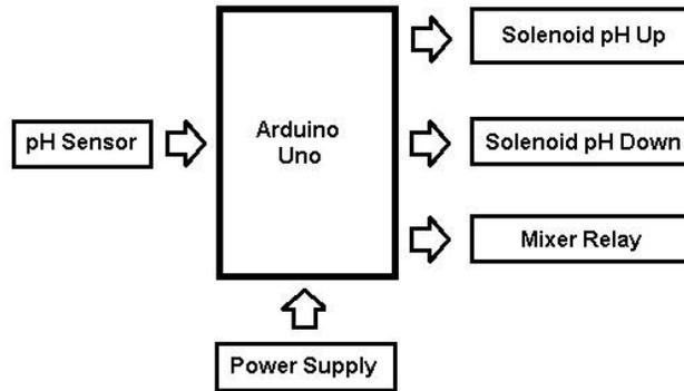
Fig. 2. Schematic Diagram The Hydroponic Nutrient PH Regulator.
