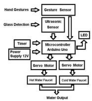
Figure 2. The proposed system block diagram.
