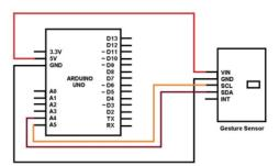
Figure 6. Schematic of the gesture sensor circuit.
