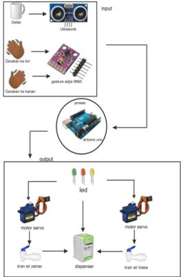
Figure 4. System architecture design.
