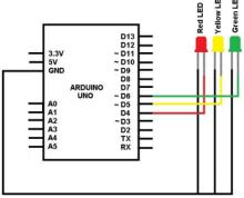
Figure 7. Schematic of the LED module circuit.
