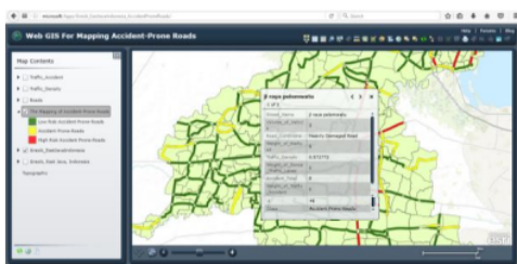
Figure 11: Classification of Accident Prone-Roads Category with Heavily Damaged Road Condition
